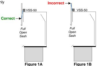
2. Install the VSS to a stationary surface located on the top of the fume hood.
