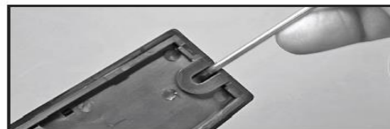
Insert Screwdriver and Pry Upwards to Remove Cover
