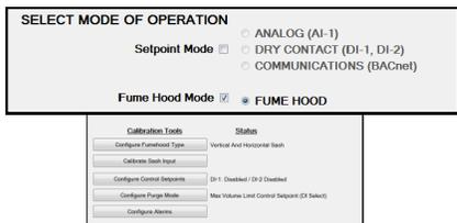
The **Calibration Tools** provided for Fume Hood Mode are accessed through a series of buttons that are positioned in the order of which they should be completed during the initial start up.
