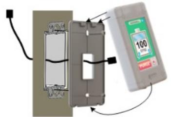
If the fume hood does not have a preinstalled electrical box available, then one will need to be installed.
