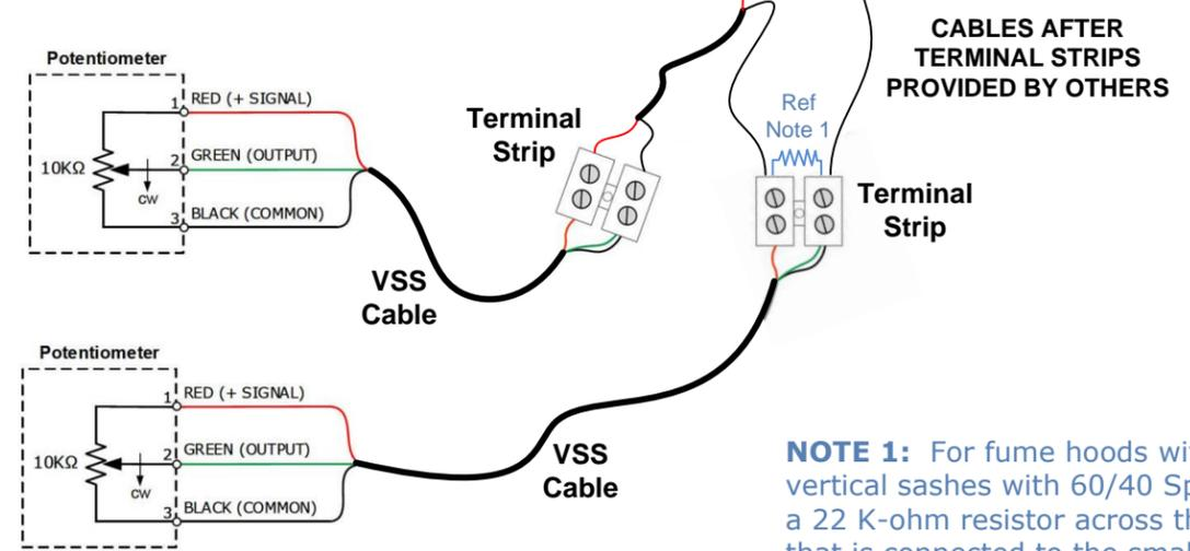
**NOTE 1:** For fume hoods with dual vertical sashes with 60/40 Split, install a 22 K-ohm resistor across the VSS that is connected to the smaller sash.
