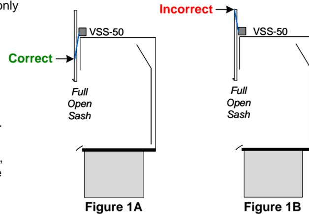
2. Install the VSS to a stationary surface located on the top of the fume hood.
