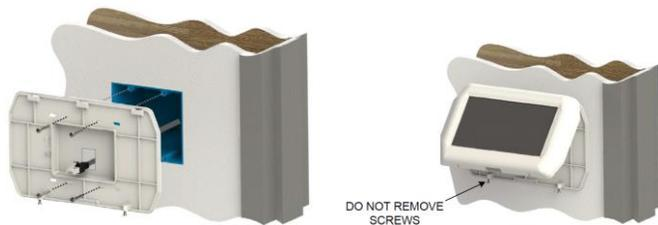
**1c. Install the Iso-Tek Sensor and Reference Probes.**
